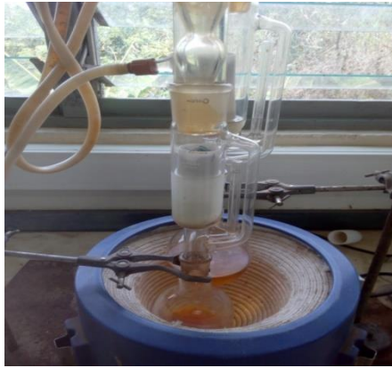
Figure 23: Soxhlet apparatus used in extracting lipid during proximate analyses of fish
