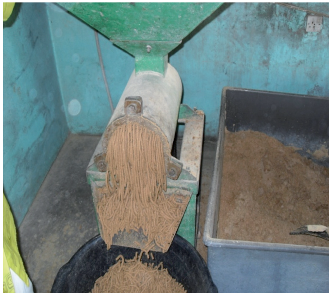
FIGURE 4 Electric fish feed pelletizer used to produce farm-made feeds
