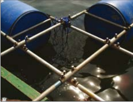
Detail of cage construction showing welded brackets forming the frame.
