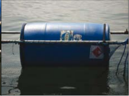
Detail showing float and net cage attachment.
