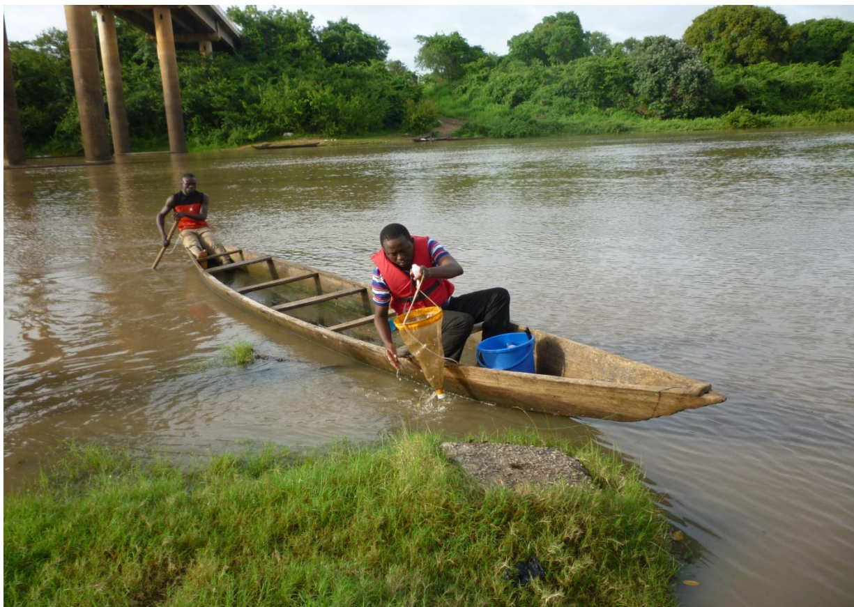
Plate A: Plankton net used throughout the study for collection of zooplankton samples at Bamboi using local canoe (picture taken, November 2012)
